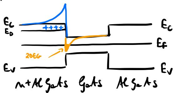
where the conduction band of Garts lies below the Fermi level, a 2DEG is accumulated. This phenomenon is called DELTA DOPING or REMOTE DOPING because the dopants (the impurities) are NOT directly in the layer where the electrons are accumulated, which means that the mobility can be extremely
